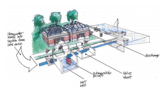
Figure 4.19 Conceptual Pump Station Schematic (Olin Studios 2012)
